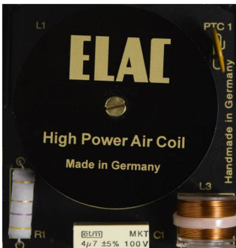
Components are used in the BS 243 Limited Edition that simply would not be feasible in a standard production run. For example, only air-core inductors are used, which cannot be magnetically saturated and therefore operate without any distortion. They are ideal for short-term extremely high loads. Peak power fidelity is unbeatable as a result.
